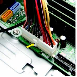
Figure 2-53 Disconnecting the main system board power connector
